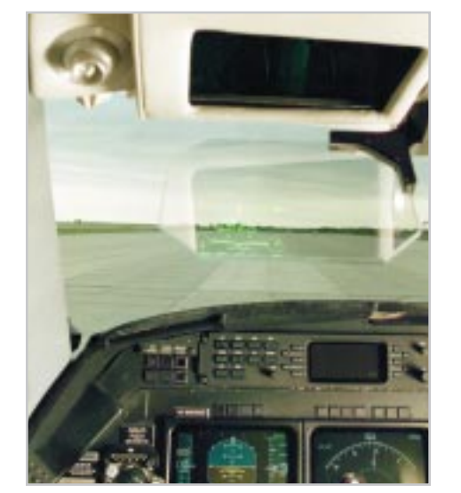
Duncan Aviation is offering G-IV operators a special package price for installation of Flight Visions' FV-2000 HUD system combined with paint and interior refurbishment. The HUD system projects flight and navigation information onto an optical glass, a "combiner," that is positioned between the pilot and the windshield.
