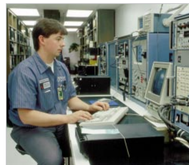
Avionics Technician Mark Cote tests a Honeywell Primus II navigation system with Duncan Aviation's computer-based test set.
