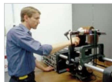
At Duncan Aviation, we always take the time to balance rotors and armatures. Here, Team Leader 1 Jim Svoboda balances a rotor from a generator.
