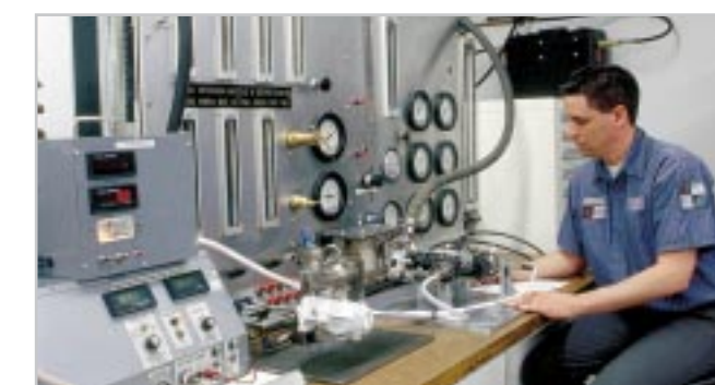
Duncan Aviation's Accessory Shop holds an STC that allows us to perform an inexpensive modification on Learjet mod valves that doubles their performance life. Jeff Witt, Accessory Technician III, is shown here testing a mod valve.
