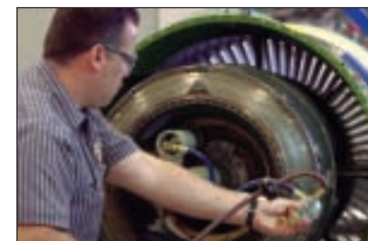
Tina Carter (left), Brian Weathers (middle) and Troy Pedersen (right) disassemble a TFE731 engine during a Major Periodic Inspection in Duncan Aviation's Engine Service Center.
