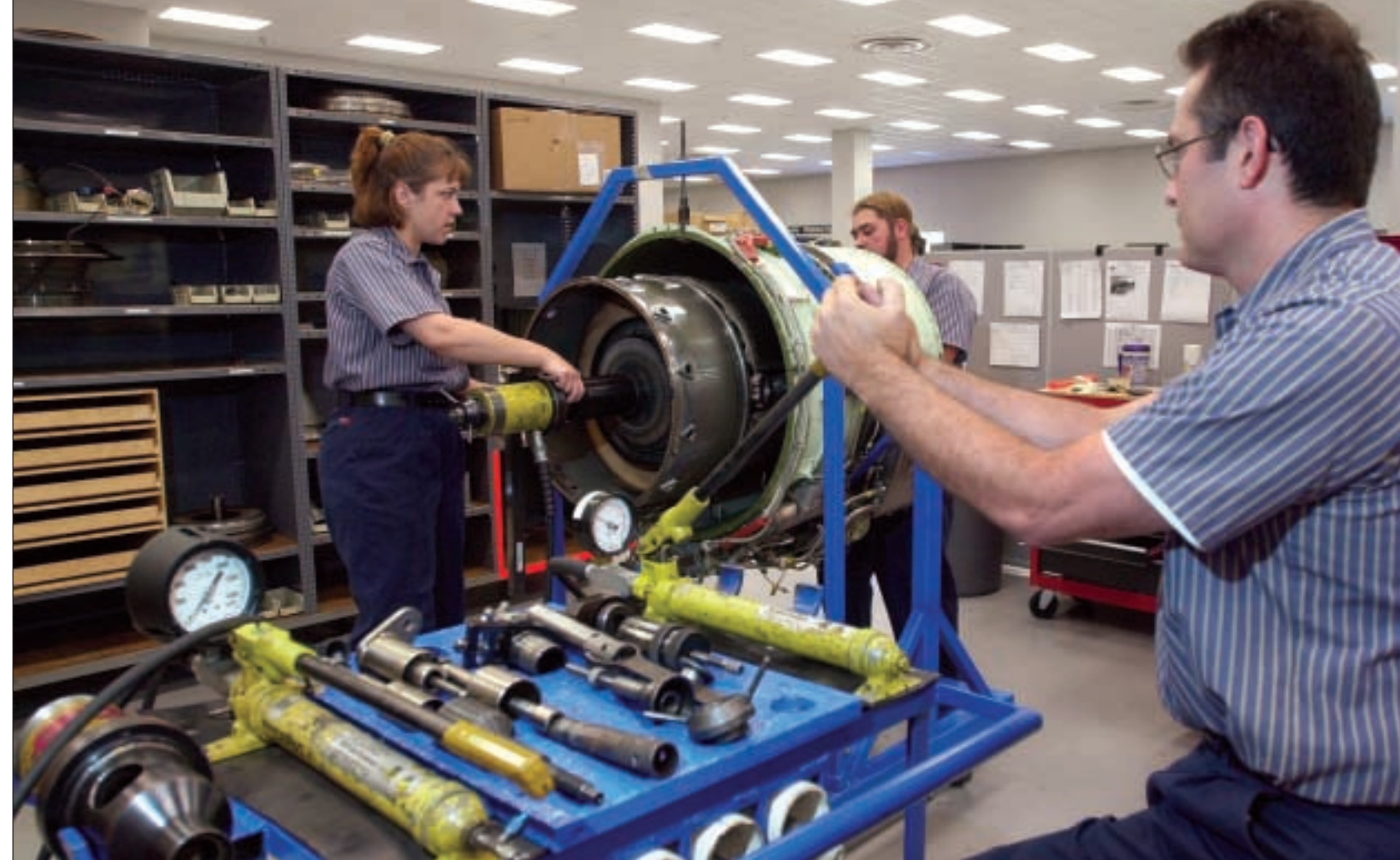
Tina Carter (left), Brian Weathers (middle) and Troy Pedersen (right) disassemble a TFE731 engine during a Major Periodic Inspection in Duncan Aviation's Engine Service Center.
