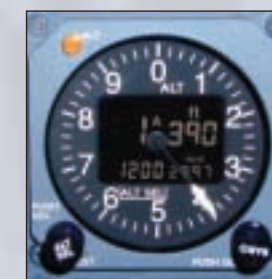
(Below) IS&S altimetry is a key ingredient for Duncan Aviation's affordable RVSM solution for the Challenger 600 and other airframes.
